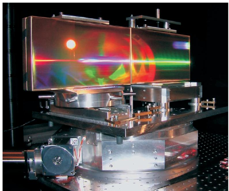
A photograph of the Phased Array grating system developed at the FSU as part of the OTTER programme.
