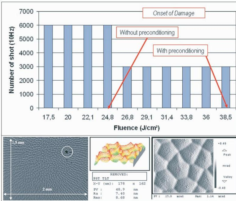
An example of a Sol-gel anti-reflection coating on an Yb:YAG substrate (LULI) and its test performance (CEA). Pre-conditioning the coating leads to an increase in the damage threshold to beyond 30 Jcm<sup>2</sup> for 10 ns duration pulses.
