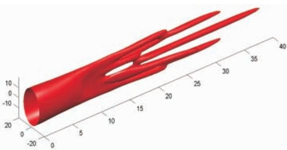
Computer simulation of an intense, ultra-short pulse propagating through a transparent medium indicating the onset of filamentation and self focussing leading to catastrophic damage.
