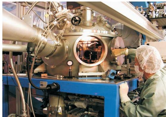
*Beam transport structure (left) and target chamber (right) used for combined heavy ion and laser experiments.*
