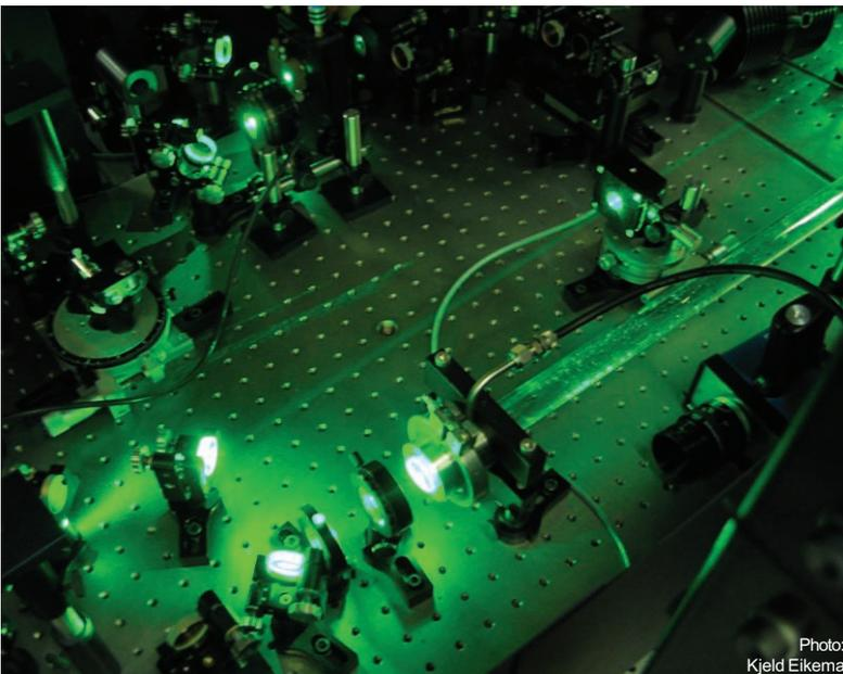
Optical Parametric Amplifier used within the FOSCIL JRA at LCVU.
