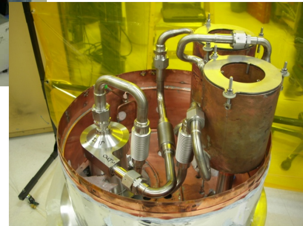
Helium circulator and heat exchangers
