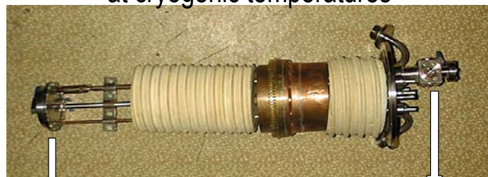
Test model of the e.-m. injector working at cryogenic temperatures
