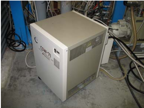
4K cryo system cooling capacity: 1.5Watts @ 4.2K cooldown time: 60min
