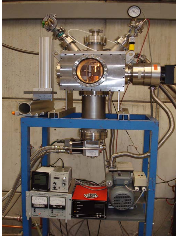
4K cryo system cooling capacity: 1.5Watts @ 4.2K cooldown time: 60min
