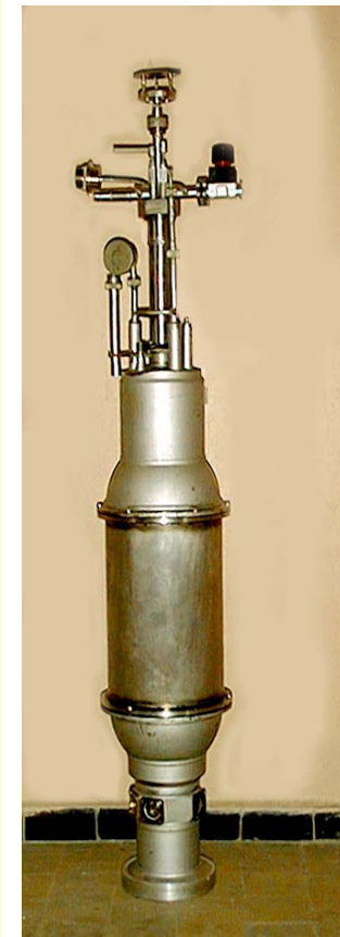
Layering module in assembly with commercial cryostat UTREX-1-RTA
