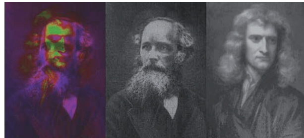
Fig. 2 | Ultrafast optical recording via self-assembled nanograting induced birefringence in fused silica. Maxwell and Newton are recorded in one image (left, in pseudo colours), however, they can be easily decoupled as Maxwell is recorded in strength of retardance (centre) and Newton in azimuth of the slow axis (right).
